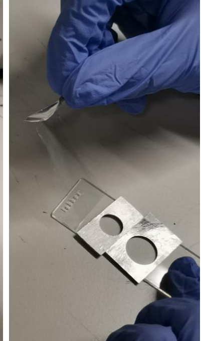
Getting a Formvar foil into target frames.
