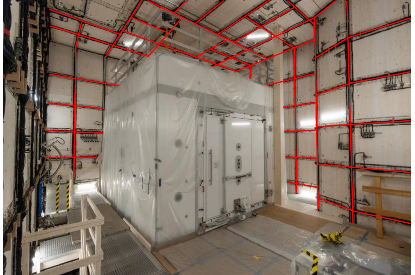
Active magnetic shield system 55km wire, kW power, mHz shielding
