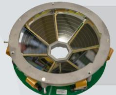
**SPIDER** modular array of Si detectors segmented into 8 annular strips (junction side).
