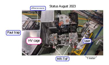
Highest energy MR-ToF device ever built! (>10~kV) Advantages for mass separation: see F. M. Maier et al., NIMA A., 1048, (2023)
