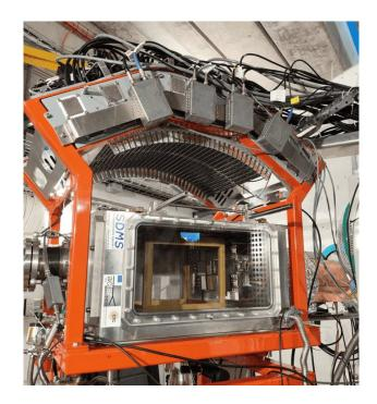
Gas mixture:  $90\% D_2 + 10\% iC_4H_{10}$  at 952 mbar
