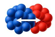
GDR can be described as an oscillation of the protons against the neutrons.
