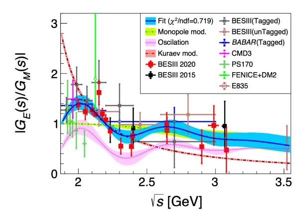
$|G_E/G_M|$  data can be well described by a function combining the monopole decrease with a damped oscillation
