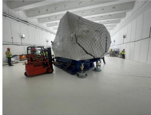
Positioning the multiplet in the L0317A hall using air cushions and a forklift for smooth and accurate placement
