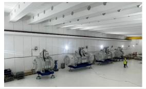
Aligning the multiplets in rows to begin preassembly tasks, with the capacity to arrange up to three lines, each consisting of four to five components, in the L0317A hall
