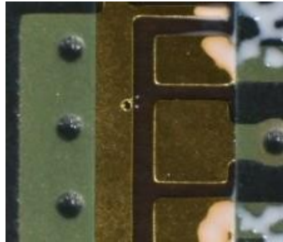
damage on wirebonding pad
