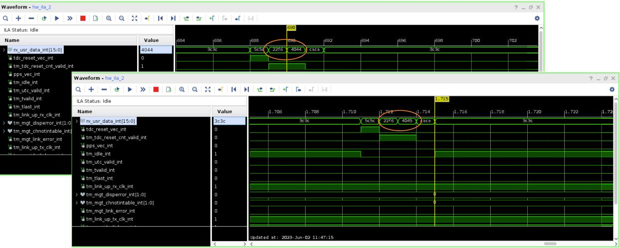
The packet structure is the one presented some time ago: 5C5C is the word that signals the TDC reset, followed by the TDC reset number and the "trigger" info. The lines below the parallel data are moved by the decoder to mark the different data.
