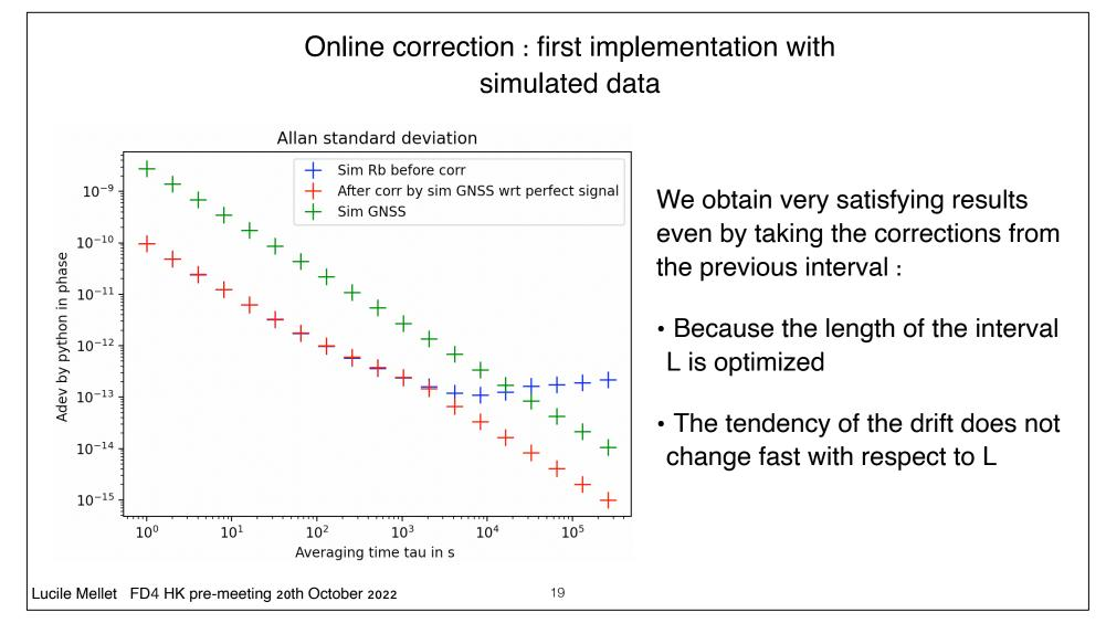
Test of the time drift correction has giving good results on simulation. The same algorithm is now applied on raw data
