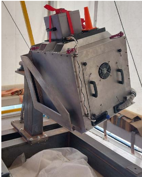
CAGIRE Close Electronics Balancing before its installation on the telescope
