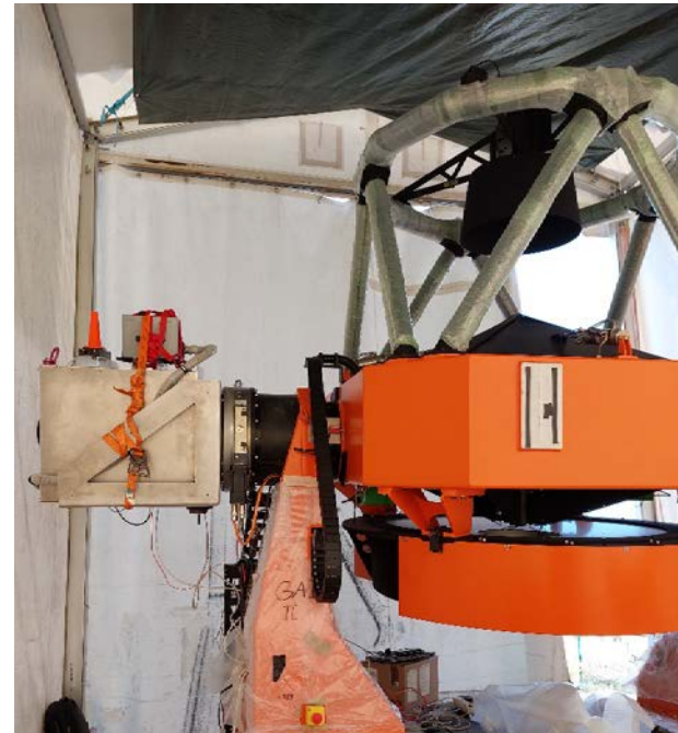
CAGIRE Close Electronics Balancing before its installation on the telescope
