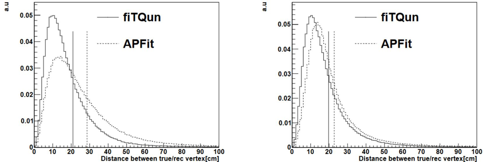
FIGURE 6.4: Single-ring electron(left) and muon(right) vertex resolution for FC true-fiducial CCQE events in atmospheric neutrino MC, compared between APFit(dashed line) and fiTQun(solid line). The resolution is defined as the 68 percentile of the respective distributions, which is shown by corresponding vertical line.
