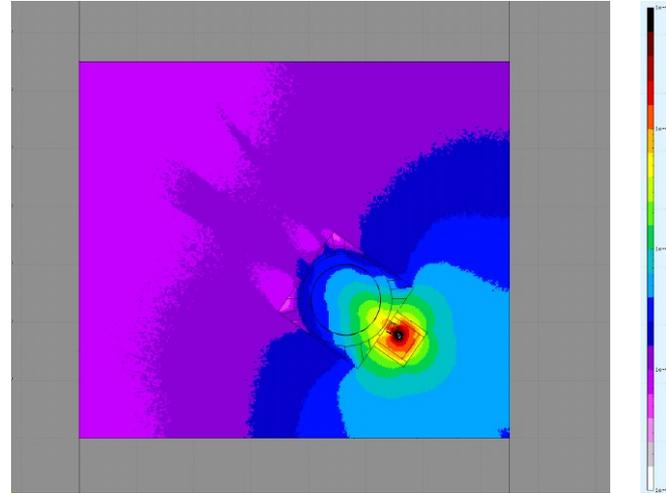
Expected neutron fluence inside the cyclotron room [Fluka]
