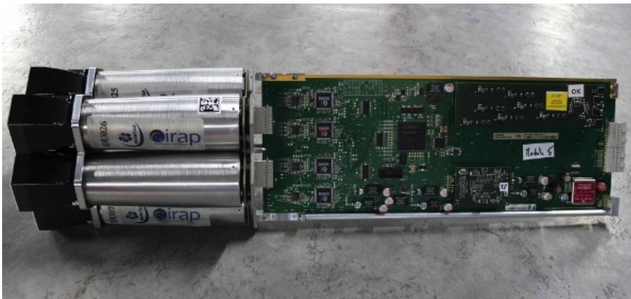
1 module of 7 Photomultiplier, credit : NectarCAM collaboration (2016)
