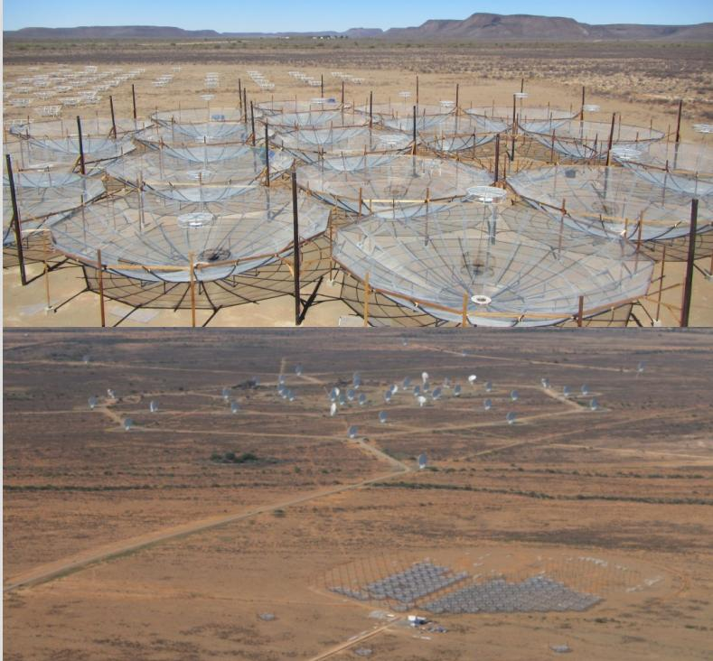
**Hydrogen Epoch of Reionization Array (HERA)** : 50-250MHz frequency band
