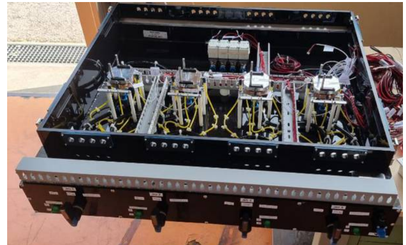
QC setup to test 4 cells in parallel with cold cycles down to -45^{\circ}\text{C}
