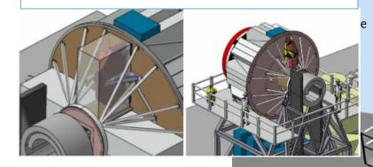
3 channel NIR spectrograph x2 Large Cryostat 130K
