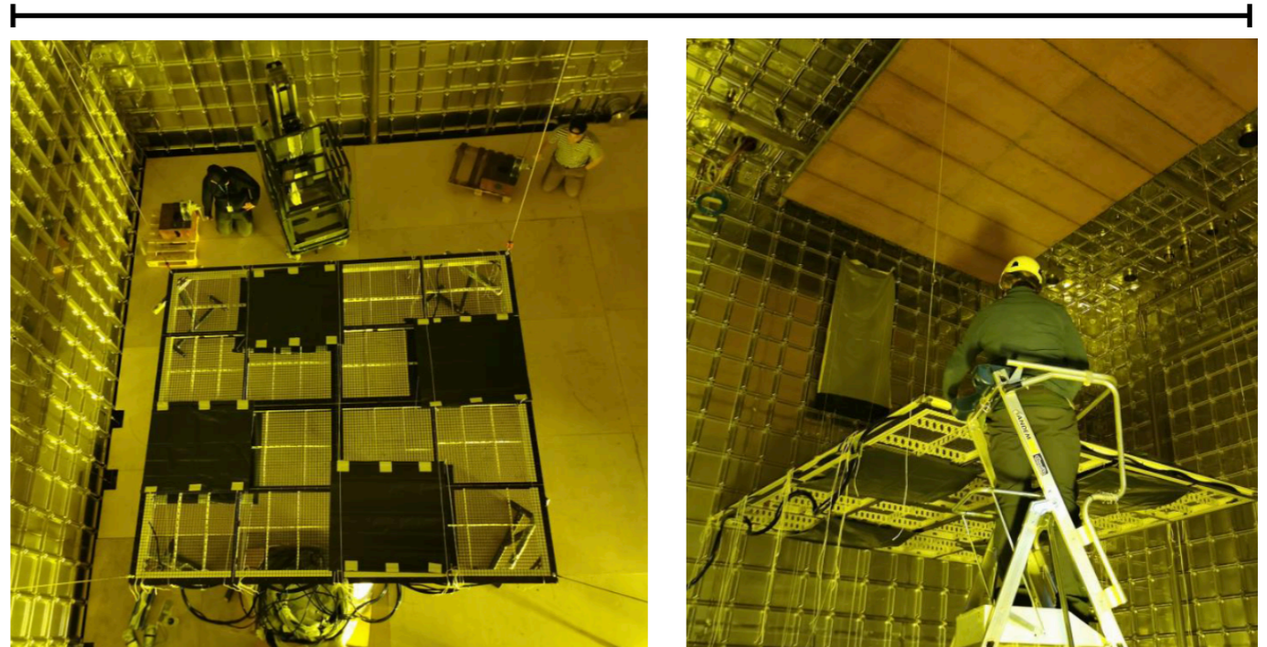
Cathode suspension below the top CRP
