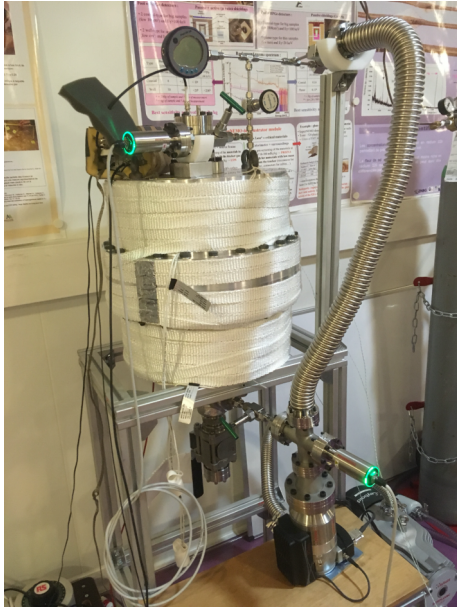
SPC-1 (2018) D = 0.4 m r_{\text{ball}} = 1 \text{ mm} (1 bar)
