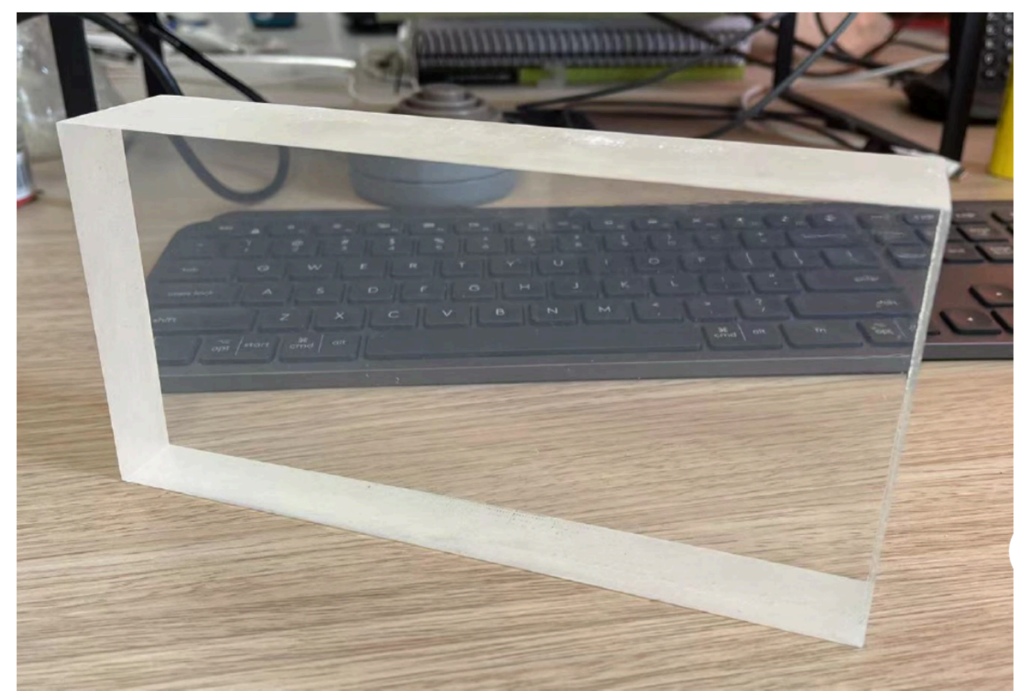
Gd(MAA) 3 doped acrylic sheet (5 cm thick)
