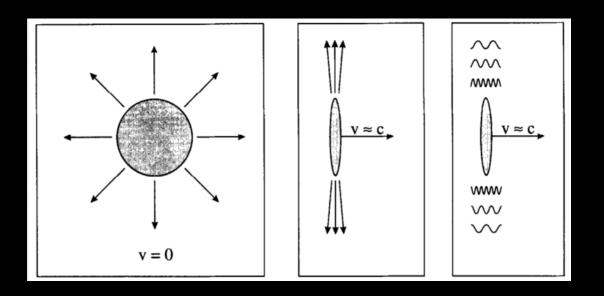
Coulomb fields of moving charges can be treated as an equivalent flux of quasi-real photons (Q<sup>2</sup>=0) which are boosted to high energies.
