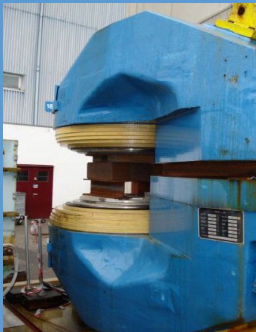
MEP48 (available at CERN), 1.5 T field over 400 mm gap
