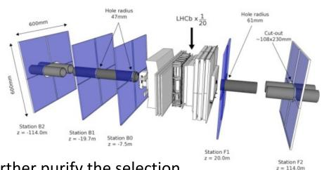
• HERSCHEL detector [JINST 13 (2018) 04 P04017] is used to further purify the selection
