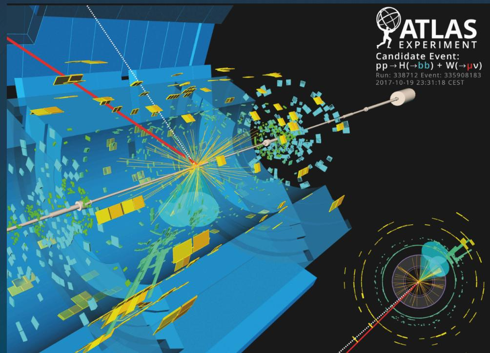
Electrons (blue) leave tracks in the inner detector, before reaching the calorimeter. Muons (red) have tracks extending from the inner detector to the muon spectrometer. Muons may leave small energy deposits in the calorimeter.
