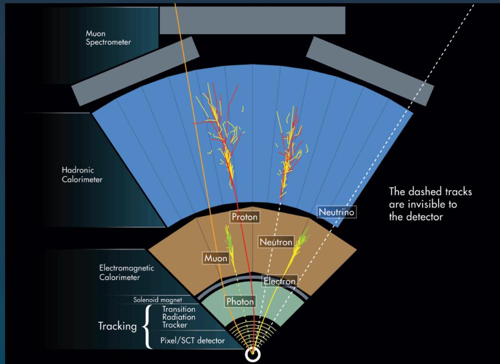
The ATLAS detector has many layers, with different types of detectors. Different particles leave behind different types of signatures in ATLAS as they travel through these layers.
