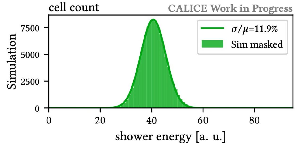
After proper filtering energy resolution in right ballpark for current prototype
