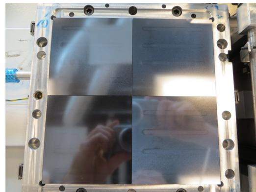
The beam test set ups consist of a **stack of short layers** built from one ASU and a readout card each
