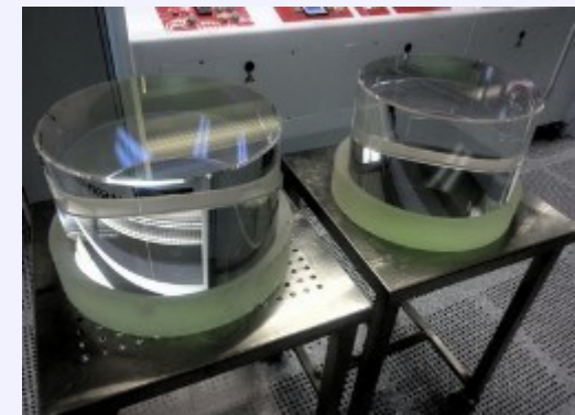
40 kg mirrors 35 cm diameter 40 cm width Suprasil fused silica
