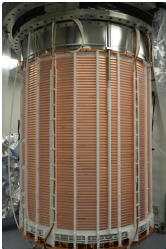
TPC: 1.5 m long und 1.5 m \varnothing 5.9 t liquid xenon in the detector (8.5 t total mass)
