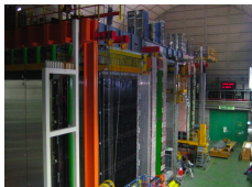
OPERA Lead + emulsion cloud chambers
