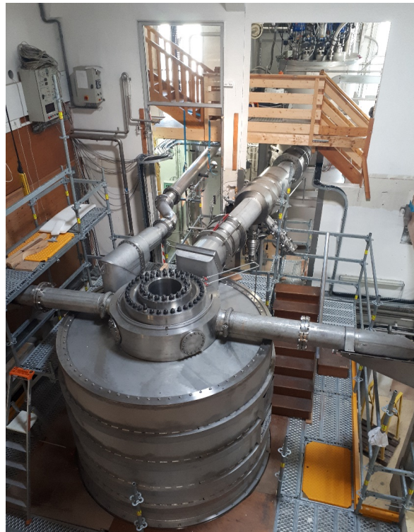
43+T Grenoble Modular Hybrid Magnet
