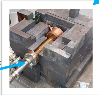
Passive shielding: 10 cm of lead around the detector.
