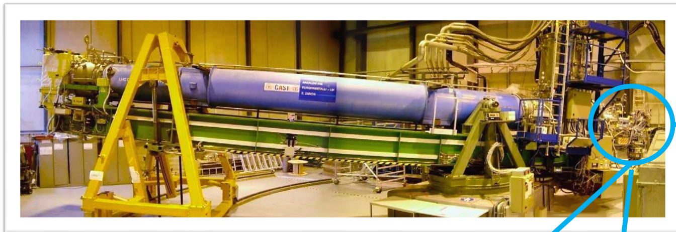
Active shielding: plastic scintillator as a cosmic muon veto.
