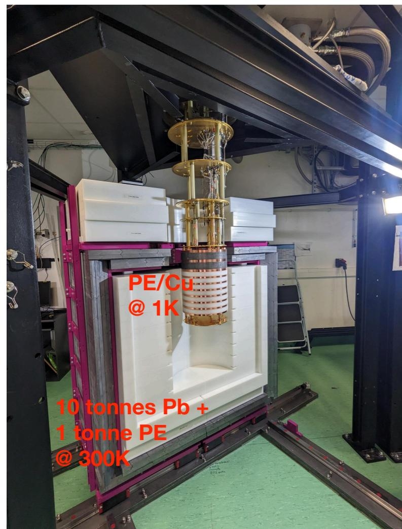
Ricochet cryostat w/ full shielding
