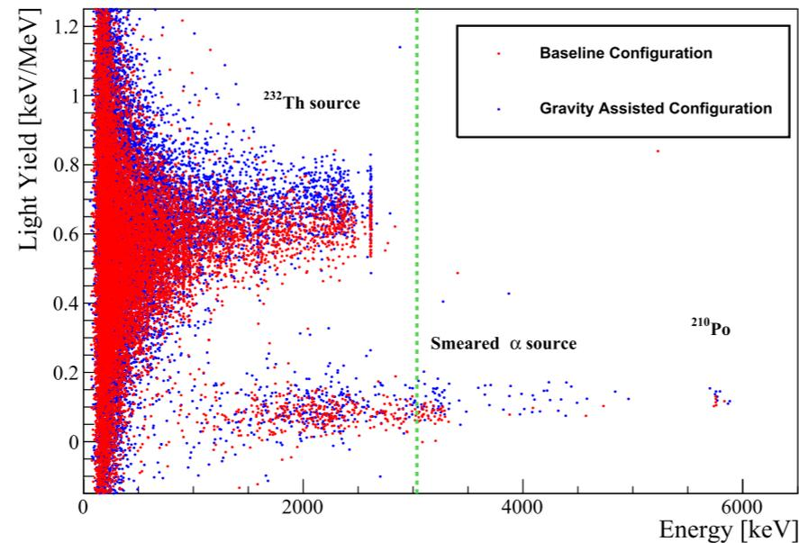
**Double readout** cryogenic detectors allows for an **evt-by-evt background rejection** :
