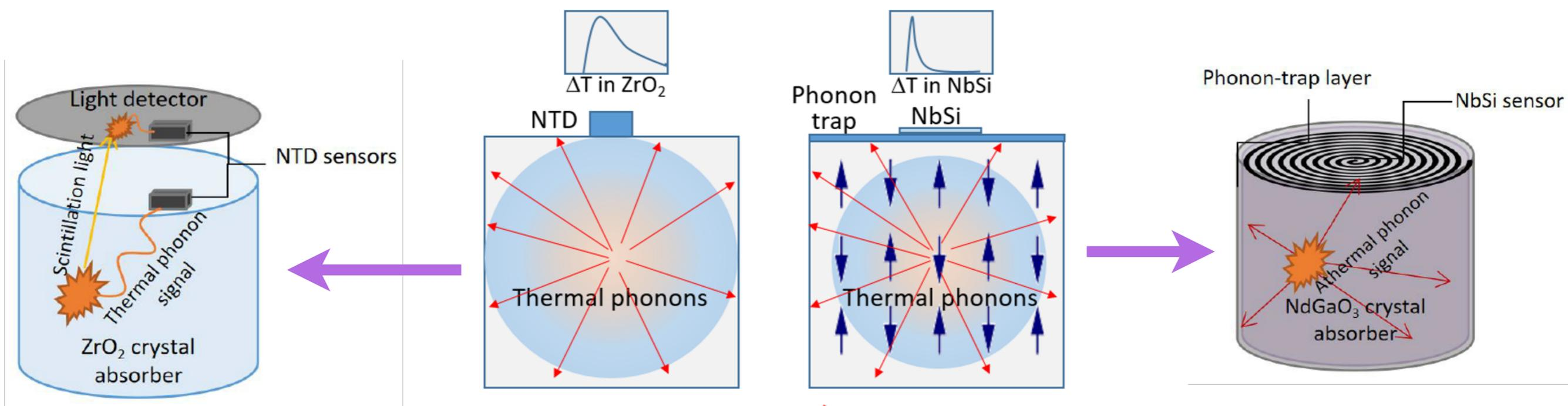
**Classical** scintillating bolometers with thermal signals
