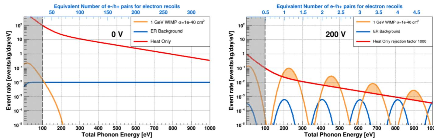
Figure 1: Response of the CRYOSEL detector operated at 0 V (left) and 200 V (right). Orange: expected NR signal for a 1 GeV/ $c^2$  WIMP with a scattering cross-section of  $10^{-40} \text{ cm}^2$ . The blue and red lines correspond to the ER and heat-only backgrounds observed in EDELWEISS detectors. The shape of the NR response is sensitive to the actual quenching factor and straggling effects for this type of interaction. In right panel a rejection factor of 1000 is considered for HO events.
