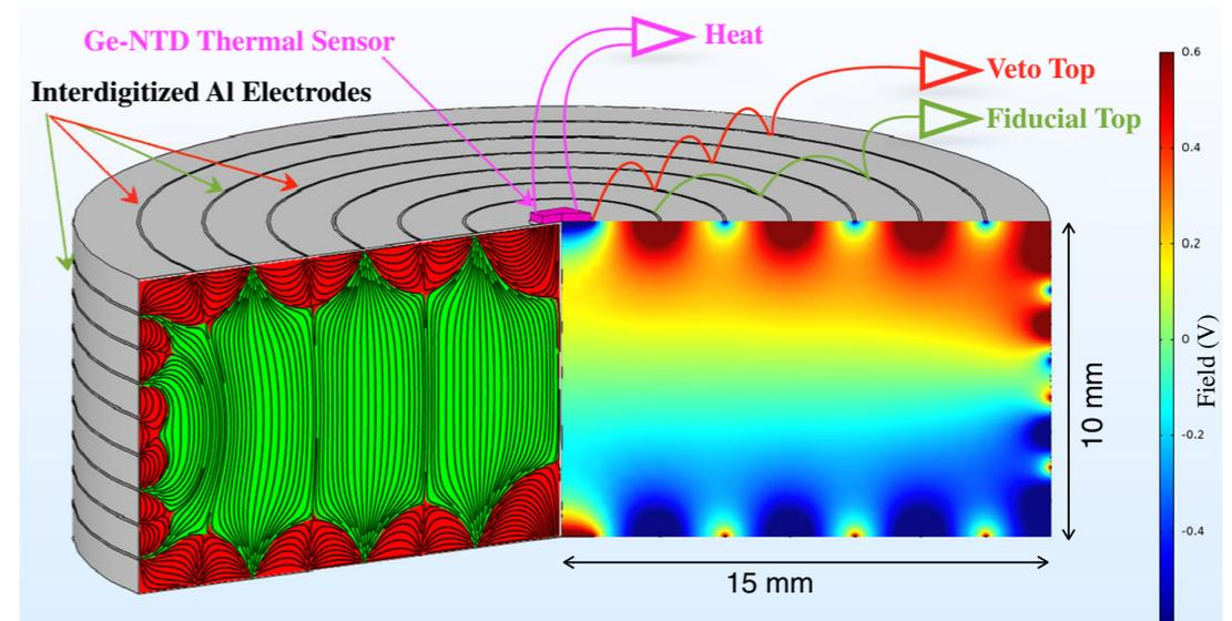
Fig. 6 Electrostatic simulation of a Full Inter-Digitized electrodes scheme on a 38 g germanium crystal ( $\Phi = 30$  g,  $h = 10$  mm). The crystal is surrounded at 2 mm distance by a chassis connected to the ground (not shown). The capacitance of the 4 electrodes with respect to the ground is about 20 pF (Color figure online.)
