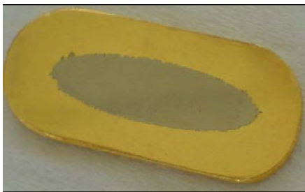
^{64}\text{Ni} electroplating on Au backing
