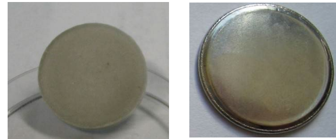
RbCl pellet before (left) and after (right) encapsulation
