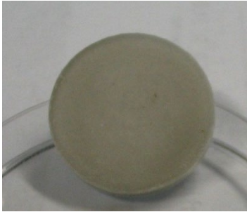
RbCl pellet (4mm thick)
