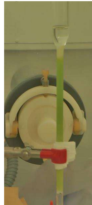
Eluting Pu by adding 0.35 M \text{HNO}_3
