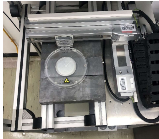
In-house made X-Y scanning system
