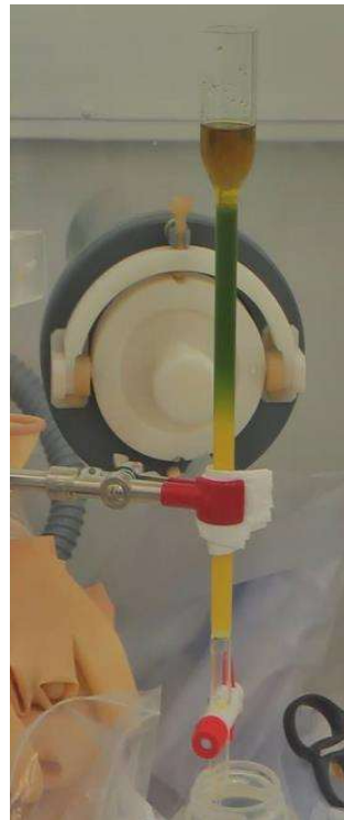
Stripping by adding 8 M \text{HNO}_3
