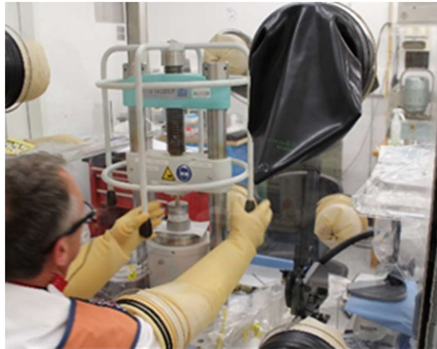
Hydraulic press in a glove box
