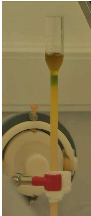
Loading Pu in 8 M \text{HNO}_3
