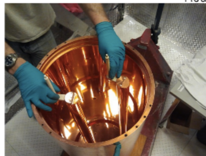
ADMX cavity tunable with metal rods
