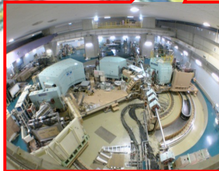
Double arm spectrometer (Grand Raiden & LAS)
