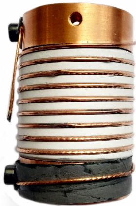
Nb 3 Sn sample on CERN type holder
