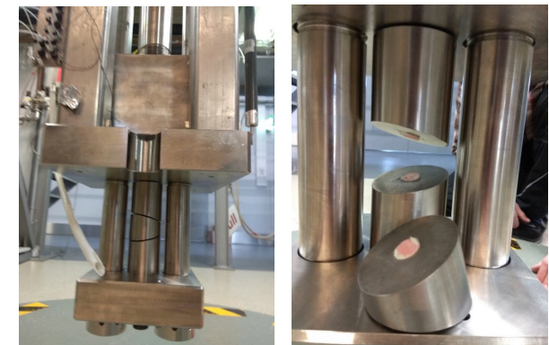
Figure 2 Compression-shear tilted test arrangement for RT and 4K test
