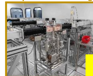
Clean room for RF Coupler conditioning
