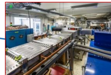
Clean room for RF coupler assembly
