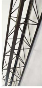
Detail of a prototype of the carbon fibre reinforced plastic (CFRP) truss to be used as a support structure
