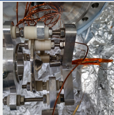
^{23}\text{Na} pellet as surface ionisation source
