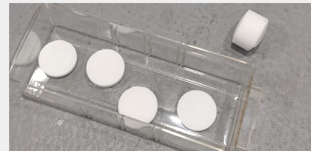
^{23}\text{Na} pellet for laser ablation source
