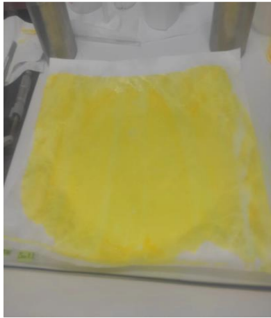
Coating the NOL film on Tyvek
