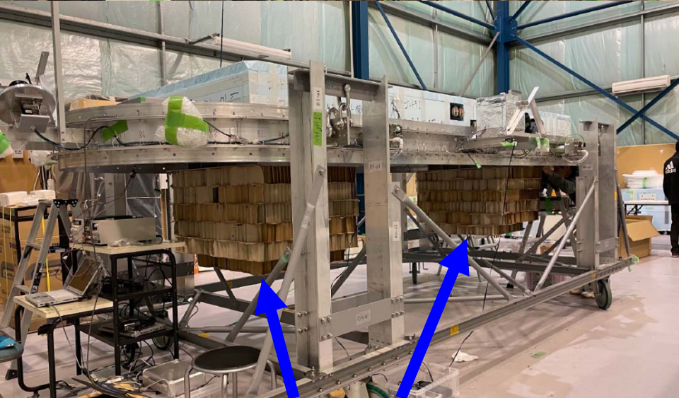
Crush Pad (paper honeycomb)
