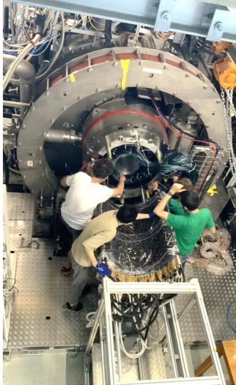
$10^8 \text{ s}^{-1}$  beamline, gradient field SC solenoid, high-rate capable low-mass  $e^+$  detectors
