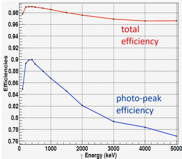
MTAS has superior g-efficiency according to GEANT4 simulations performed by B. C. Rasco (LSU)
