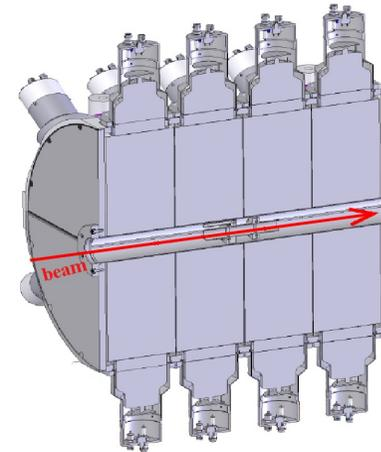
Since 2011, SuN: barrel shaped scintillator detector, divided into eight optically isolated segments. Each of the segments is read by three photomultiplier tubes,. The diameter and length of the detector are both 16 inches. The diameter of the beam line bore hole along the detector axis is 45 mm.
