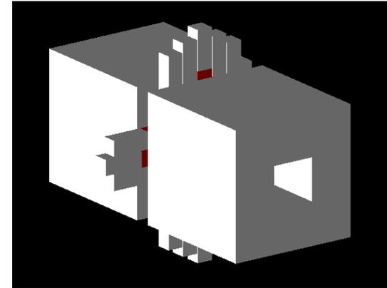
Fig. 4 : view of possible arrangement of the 16 LaBr<sub>3</sub>:Ce (red) in the middle of the NaI crystals (grey) (courtesy A. Beloeuvre).
