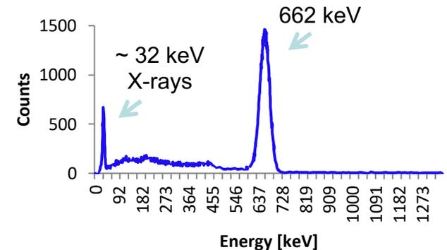
g-energy spectrum of  $^{137}\text{Cs}$  activity measured with a single MTAS module.
