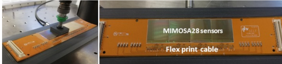
Know-how @ IPHC: light module assembly
