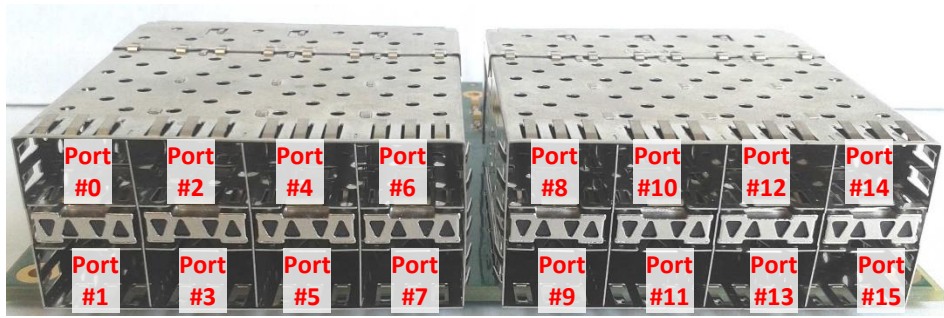
Fig. 5. Front view of the multi-SFP Mezzanine Card.
