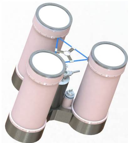
3-receiver cryostat sharing one cryogenic system
