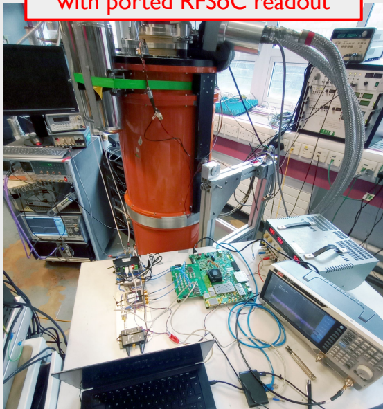
Reading out prototype KID array with ported RFSocC readout
