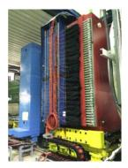
• MUV3: 50 mm thick scintillator tiles, placed behind an EM calorimeter, and hadronic calorimeter and an iron wall, used for muon identification
