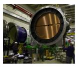
• LKr: electromagnetic calorimeter filled with about 9000 l of liquid Krypton at 120 K
