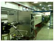
• GigaTracker: silicon pixel spectrometer with very good time resolution, reconstructs properties of incoming beam particles (K+)
