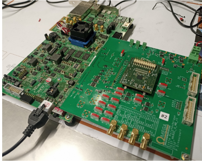
Figure 19: Test board used at OMEGA, LLR and IRFU to perform all the HKROC tests. The ASIC is mounted on a mezzanine board, itself mounted on a mother board connected to a KCU test board.
